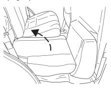
2. Rotate seat cushion down into the seating position making sure that the seat cushion is locked into place and that the safety belt buckles are exposed.
